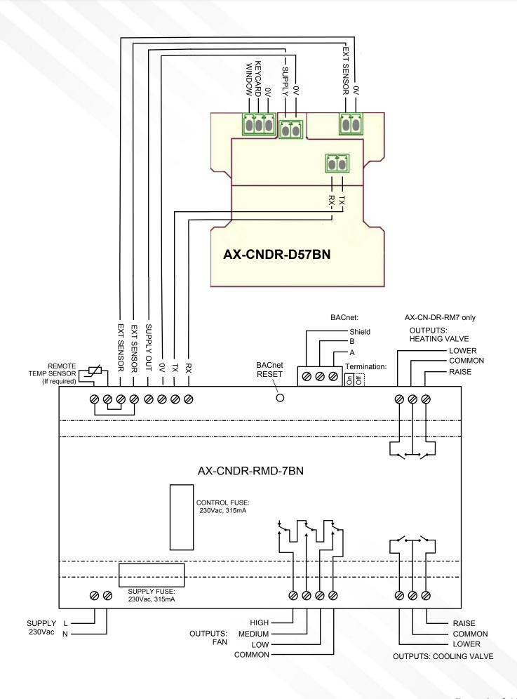
Digital Room Controller with BACnet and Relay modules
