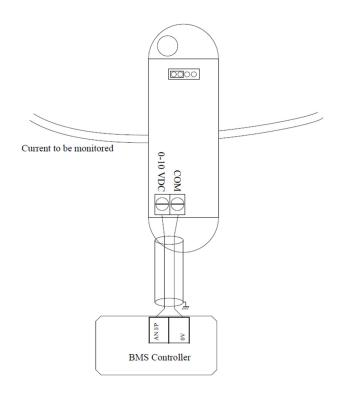
As a general rule screened cable should be used to connect signal to a BMS or other controller. The shield should be connected to the earth at one end only.
