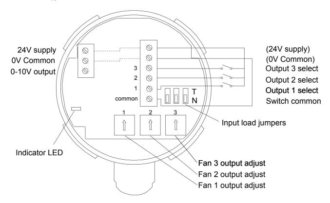
With none of the inputs selected, the output will be 0V.
