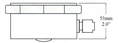
The AX-GS-CM-V-65 provides a side-entry M20 cable gland as standard, whilst the -R version offers the option of rear cable entry allowing the unit to be mounted to a wall with its cables hidden from view. The -R version is supplied with a M20 gland plug and gasket that can be repositioned to the side or the rear.
