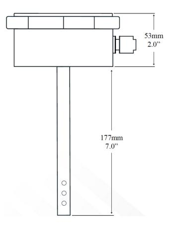
0-300ppm with duct probe
