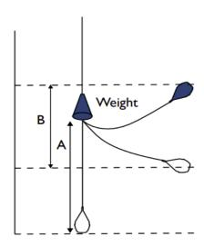
The height at which the float hangs and the distance of the cable weight from the float can be adjusted. The differential between the start and stop levels is at its lowest when the cable weight is about 10 cm from the tip of the float's strain-relief.
