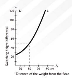
The switching height differential is adjusted to the required level by means of the cable weight. Curve B shows the start-and stop-height differential of the Float Switch in relation to the distance of the weight from the float.
